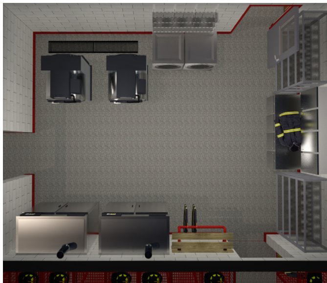
The laundry area of a firehouse should include a washer/extractor that's designed for PPE and a high-temperature residential washer for suitable PPE and personal clothing.
