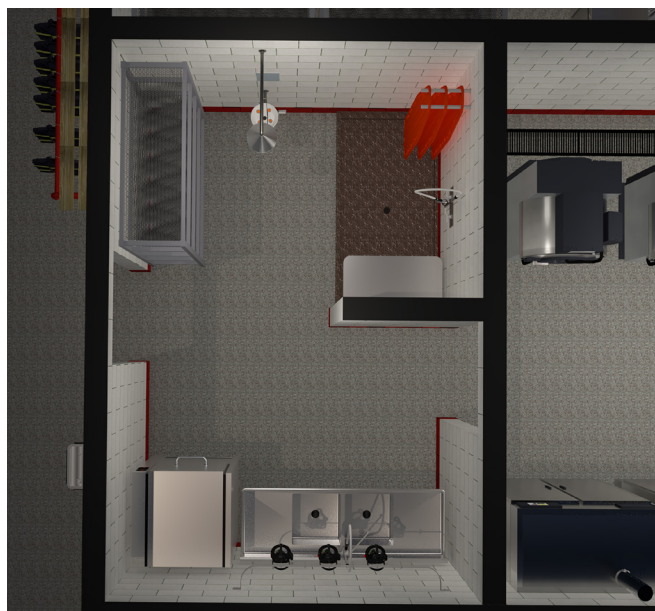
Gross decon area elements are metal shelving, a tub sink and a gross decon chamber.
