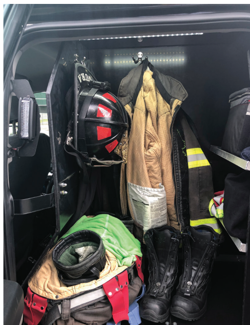
Pictured here is a command vehicle PPE SCBA locker, installed behind the driver's seat in the cab of the truck. Notice the SCBA is located behind the bunker coat in a secured bracket.
