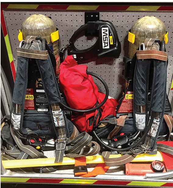
Coral Springs-Parkland Fire Department has placed its SCBAs and firefighting equipment in outside cabinets to keep contaminants out of cabs. Photo courtesy of Coral Springs-Parkland Fire Department
