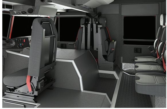
Flat surfaces, devoid of nooks and crannies, makes debris removal inside cabs easier for firefighters. Spartan Motors
