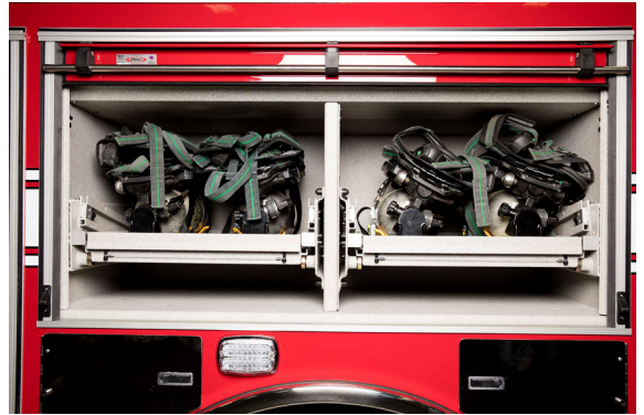
Roll-out shelves for gear and SCBAs makes it convenient for firefighters to leave contaminated items out of cabs. Pierce Mfg
