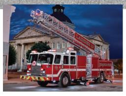
extruded aluminum body has a SideStacker hosebed and storage for 156 feet of ground ladders. With a wheelbase of only 235 inches and a short rear overhang, this rig provides impressive maneuverability. The fire package includes a 1,500-gpm Hale DSD pump and a 500-gallon UPF Poly III water tank. The 100-foot aerial features a 2.5:1 structural safety factor and crisscross under-slung outriggers with an 11-foot jack spread.
