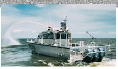
Inc. The Endeavor 38-foot vessel includes upgraded side-sonar scan for search and rescue support, remote fire monitoring on the roof, and patient transport equipment. It features a full walk-around cabin with easy bow access, shock-absorbing seats and triple Yamaha 300-hp outboards. It also has a Darley LSDE 1,000-gpm pump and a 300-gallon water tank. silverships.com
