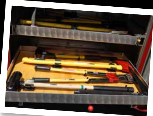
The clear width of compartment openings should be determined when laying out equipment mounting inside of slide-out trays. Note the efficient use of space to mount the forcible entry tools.
