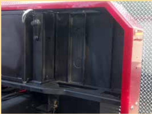
The underside of a fabricated steel front bumper. Note the front and side supports to reinforce this area. This style of bumper will protect the crew and rig in the event of a frontal collision. Photos by Tom Shand
