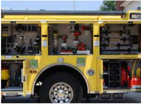
High side body compartments can have pegboard or similar material provided in the reduced depth sections to permit mounting of hand tools and appliances.
