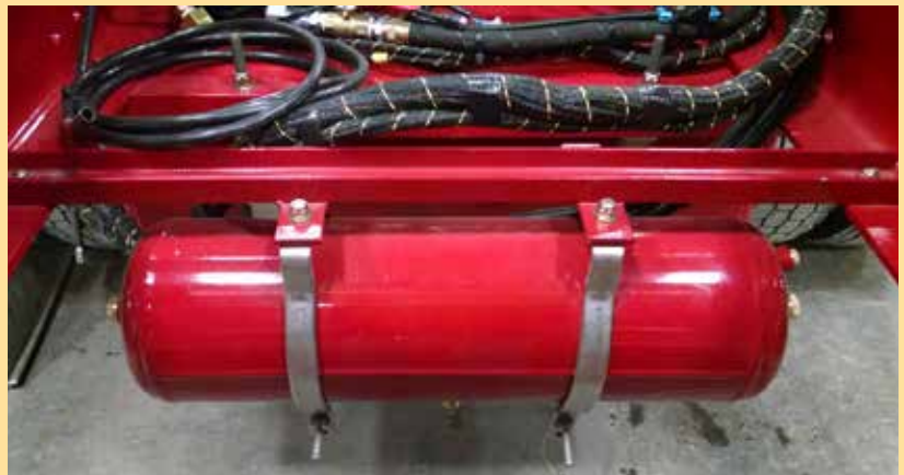
Finish painted frame rails along with stainless-steel straps and hardware on chassis components will resist rust and corrosion in these important areas that are often overlooked.
