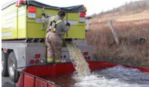
Tankers/tenders must be capable of being emptied or at the rate of 1,000 gpm, at a minimum. Photo by Jay Bradish
