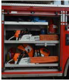
A combination of slide-out trays, fixed shelves and modules provided space for ventilation equipment on this San Diego ladder truck.
