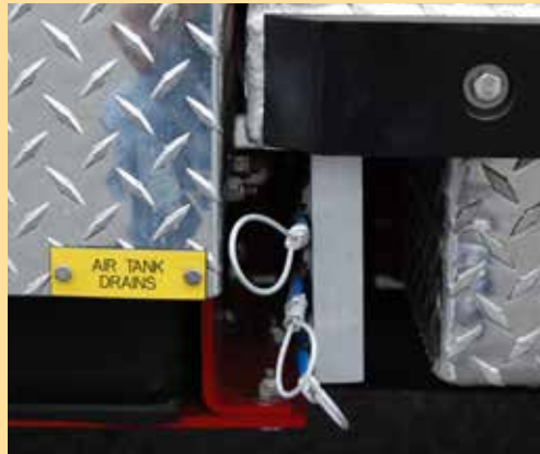
Chassis air reservoirs should be provided with remote cables that permit personnel to regularly drain tanks.
