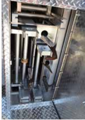
This shows an efficient use of walkway storage on this heavy rescue for roof hooks, 16-foot roof ladder, 28-foot extension ladder and small attic ladder.
