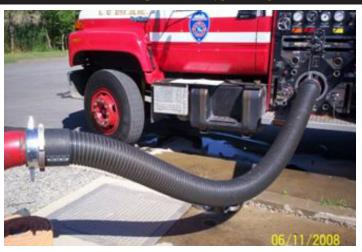
Start the apparatus and engage the pump. Prime the pump by bringing the RPMs up to 1,100. Activate the primer valve and operate the pump as you would during drafting operations. Document the amount of time it took to prime and start flowing water. The acceptable time for a 1,250 GPM pump is 30 seconds or less.
