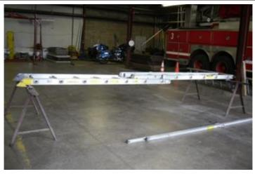
major difference is the weights that will be used. Once the ladder is correctly mounted on the saw horses and the board is positioned, 250 pounds of weights is used; the weight is the same for both time periods during this test.
